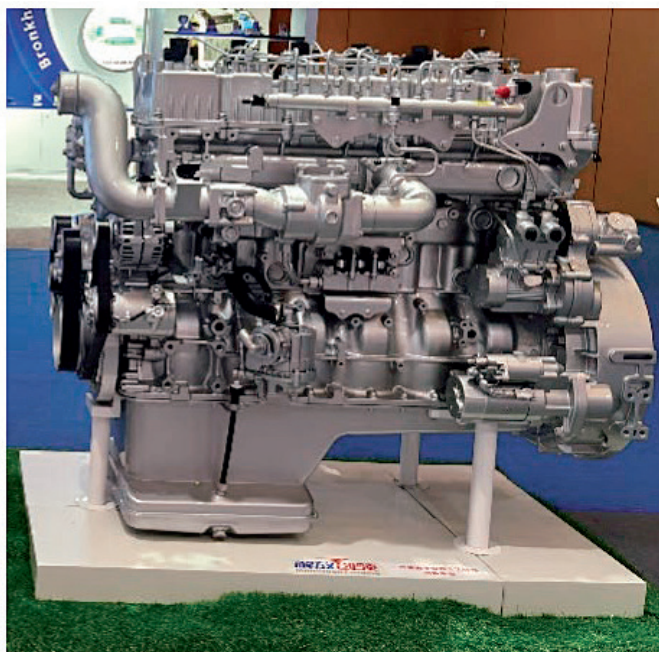
Fig. 3-1-64 Ammonia-Hydrogen Synergy Fuel Direct Injection Zero-Carbon Internal Combustion Engine System.
